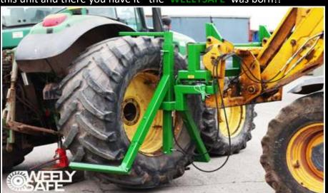
It is <u>Clean, Simple</u> and <u>Safe</u> to use, enabling the operator to remove, carry, store & refit most large tractor / combine wheels & tyres up to 2m in diameter (2.3m with an extra adaptor) either in a yard or even field situations. It will fit most tractor loader machines and telehandlers. With ever increasing wheel sizes and lone working situations, it is a must for every farm.
